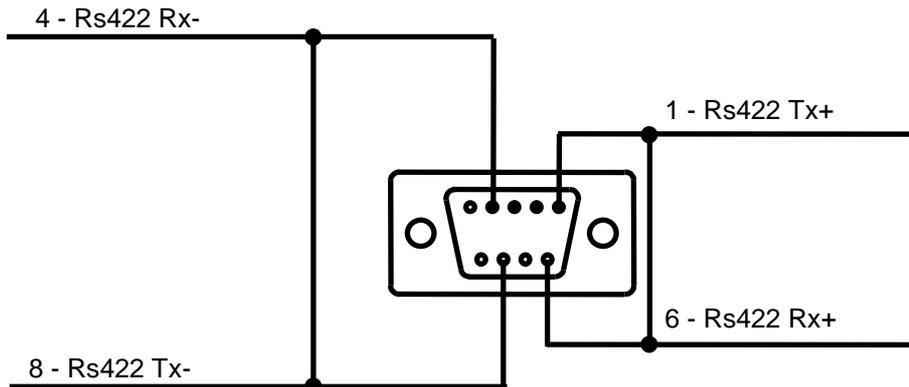
Maybe you'll need to do a short circuit between pins 2 and 4 on printer side connector, in order to enable the line terminator resistance (already included on the cpu board).
